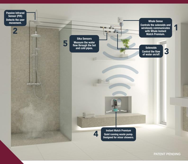
Whale Sense is a solenoid\* controller designed for the bathroom which reduces the risk of flooding.
